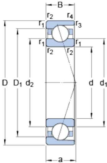
71964 ACDMA/HCP4A Bearing 2D drawings and 3D CAD models
